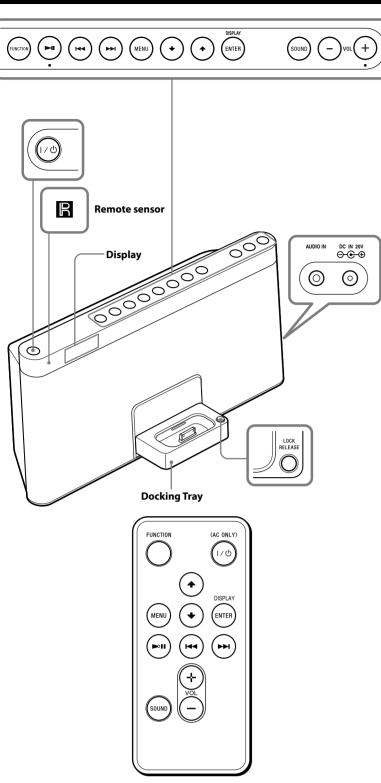
**VOL** + and ►**II** on the unit and the remote commander have a tactile dot.
